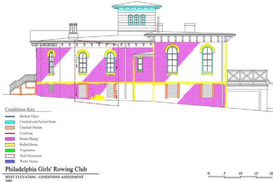
Drawing 10: West Elevation, Conditions Assessment (AutoCAD drawing by author, 2005)
